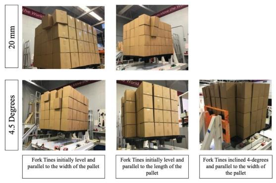
Figure 7: Representative photos displaying unit load instability during vibration testing
