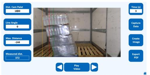
Graph 5. Max deflection on transport identified and measured by artificial vision system.
