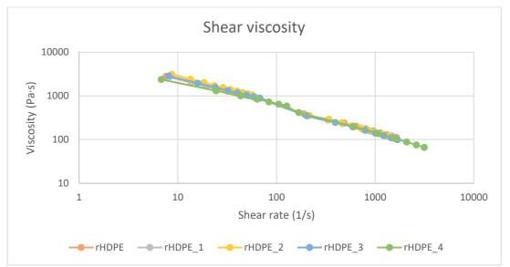
Figure 3 Shear viscosity of the different formulations
