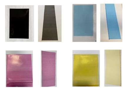
Figure 1 Colour obtained after printing on PLA (each colour left) and cardboard (each colour right).
