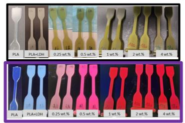
Figure 6 Injected specimens of LDH nanopigment compounded with PLA LX175.
