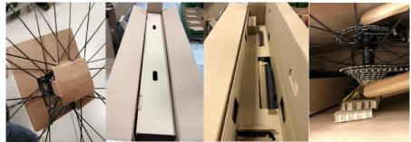
Figure 3. Protection and immobilisation components detail of the physical prototype
