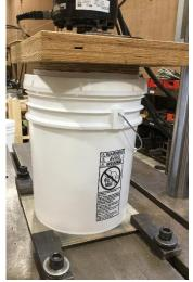
Figure 1. Experimental setup for the pail compression testing on a rigid surface
