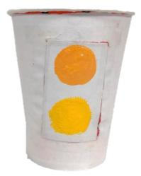
Figure 1. Shows the color change from yellow to orange-red of the thermochromic label when a hot liquid is poured into a cup.
