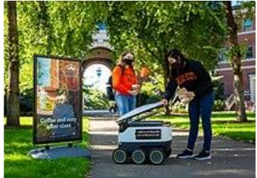
Figure 1. A sidewalk robot made by Starship is shown delivering food to students at Oregon State University campus
