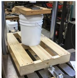
Figure 3. Experimental setup for the pail compression testing on a flexible, pallet segment using the center support location
