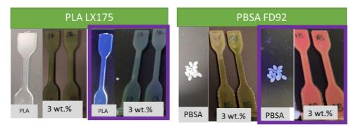
Figure 5 Injected specimens of MMT nanopigment with PLA and PBSA at 3 wt.%, and blanck samples for control
