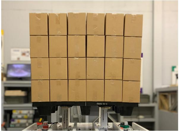
Figure 3: Representative photo of the unit loads used to conduct the dynamic fork tine support experiments in the parallel to the width orientation
